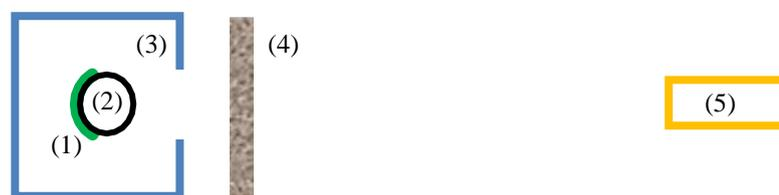
Fig. 1. Experimental setup for attenuation measurement (not in scale): (1) plaque, (2) eye phantom, (3) Pb diaphragms, (4) attenuation layer, (5) detector.
