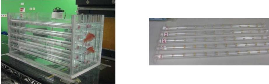
Figure 1 Water phantom ( $60 \times 30 \times 30 \text{ cm}^3$ ), and pipes filled with RPL dosimeters
