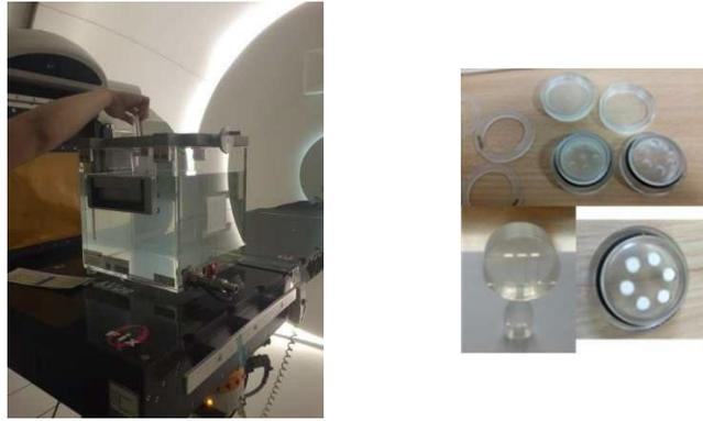
Figure 4 PTW water phantom and holders for alanine, TLDs, RPLs and OSLs alanine dosimeters
