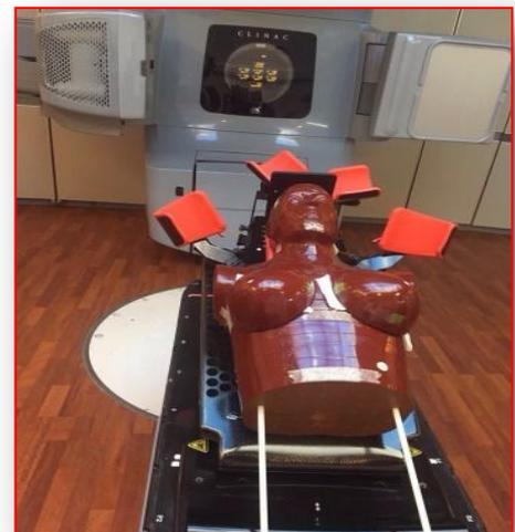
The same plan was used for all patients. Two opposite tangential beams were created, one medial and the other lateral to the breast or chest wall. Each beam is of 50% weight; 30° motorized wedge was inserted to the beam field. The beam energy used is 6 and 15 MV. The prescribed dose was 50 Gy divided over 25 fractions each of 2 Gy.
