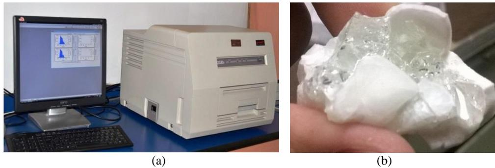
FIG.1. (a) Harshaw 4500 equipment, (b) synthetic  $\text{CaSiO}_3$  polycrystalline.
