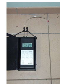
Pressure measurement below slab P1, P2, P3
