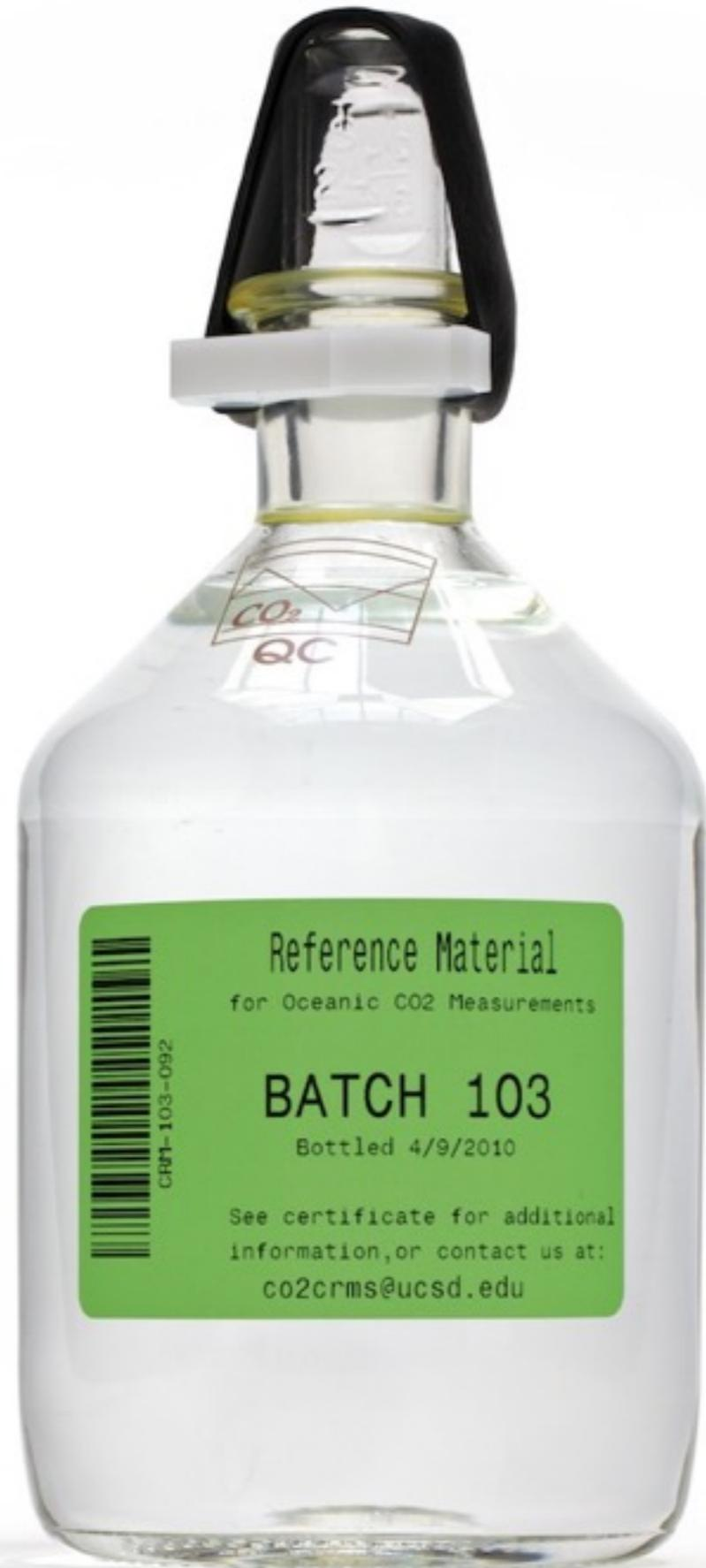
**Closed pyrex bottle with air-tight seal**
