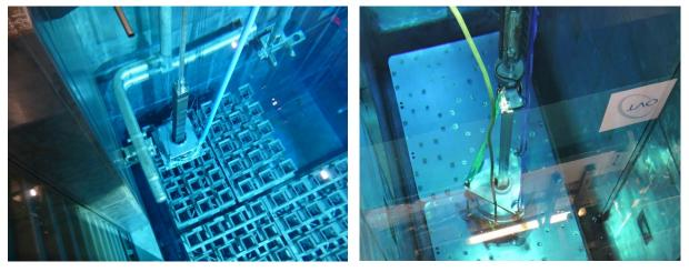
Figure 2&3. PGET is performing spent fuel verification of the PWR fuel (Ringhals) and WWER-440 (Loviisa)
