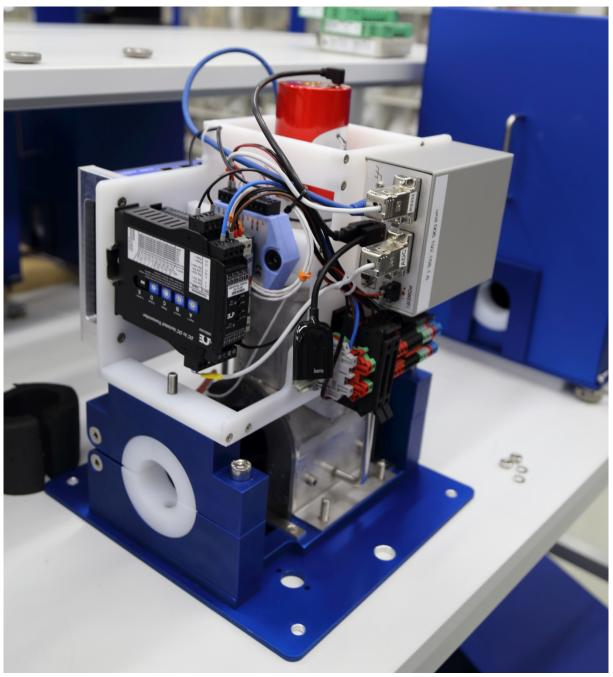
Figure 3. Under the hood of the On-Line-Enrichment-Monitor (OLEM)
