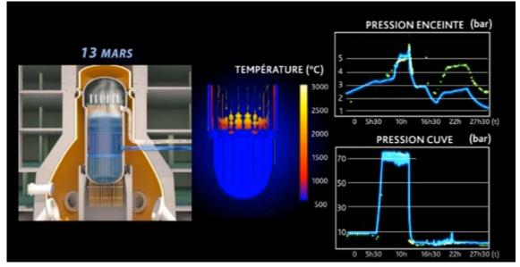
Figure 2: Simulation for Unit 1
