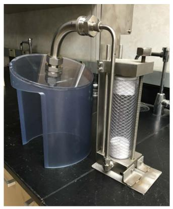
*Figure 1: Prototype of the ruthenium scrubber for On-Site Laboratory (OSL) (Ruthenium Absorber Scrubber Project: RASP)*
