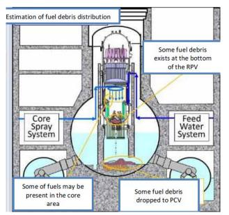
Figure 3: Estimation of fuel debris distribution in Unit 3 © International Research Institute for Nuclear Decommissioning
