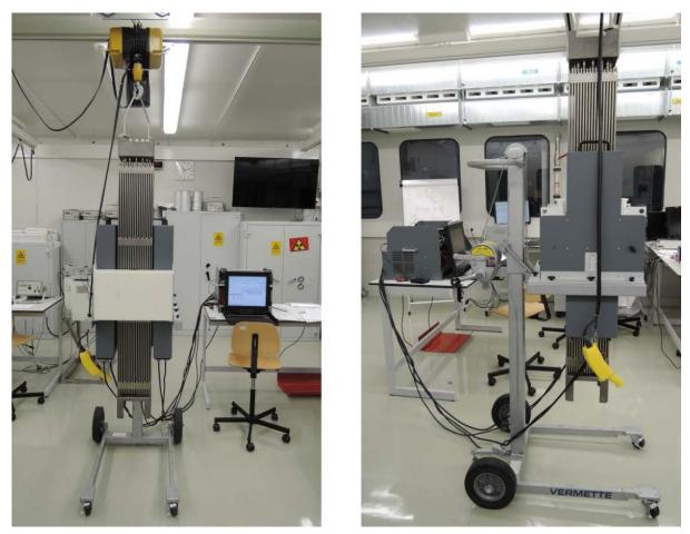
*Figure 4&5. Fact Neutron Coincidence collar is undergoing performance evaluation on the fuel containing burnable poison rods*
