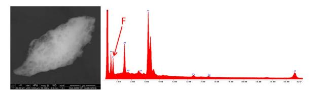
Figure 2: Scanning Electron Microscope (SEM) image and associated nergy Dispersive X-Ray Spectroscopy (EDX) spectrum of an uranium-bearing particle in which fluorine was also detected
