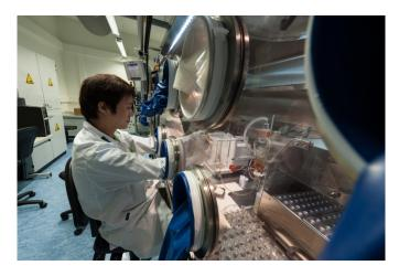
Figure 2: A chemist aliquots a small weighed quantity of mixed uranium – plutonium solution into a penicillin vial under glove box conditions. Each vial is an in-house reference material, and will be used later by the IAEA for verification of spent fuel samples
