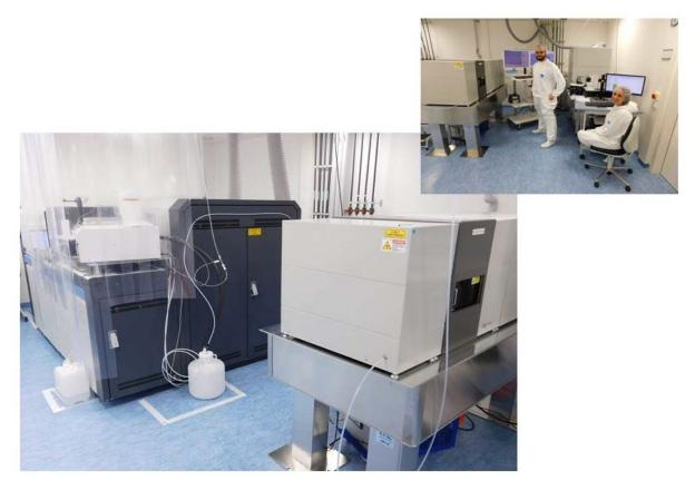
Figure 1: Femtosecond Laser Ablation System coupled to MC-ICP-MS for the analysis of particles and other solid matrices
