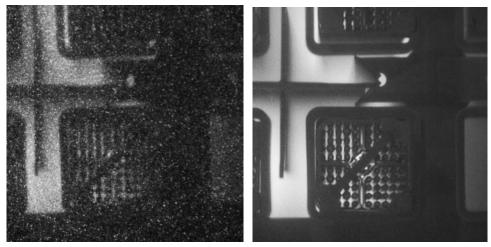
Figure 3. Image seen through a Cerenkov viewing device, before and after image processing
