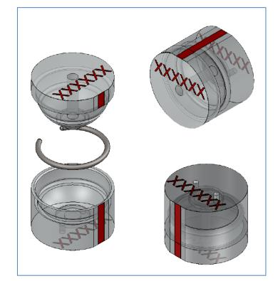
Figure 1. Latest design of the Glass Seal (GLAS) with a new self-aligning round bottom avoiding breaking on closure
