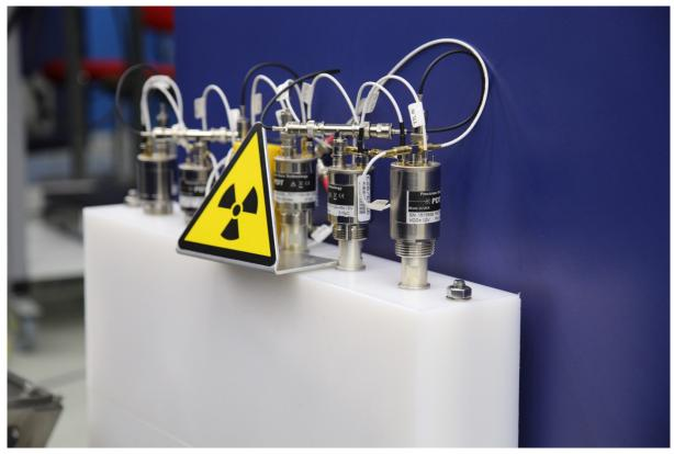
*Figure 2. Neutron slab detector for testing alternatives to He-3 filled proportional counters*
