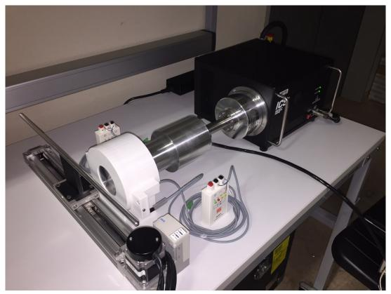
Figure 2: Testing of the fuel rod scanning system prototype
