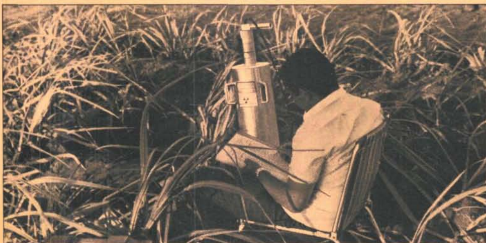
Below: A neutron probe in use during soil investigations under IAEA's Technical Assistance in the Gezira region in the Sudan. Photo: Cope
