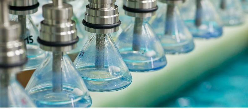
Oxygen isotope fingerprints of water give information about its origin and age, and they are measured by equilibrating water samples with CO<sub>2</sub> gas in the laboratory using mass spectrometry. (Photo: IAEA)
