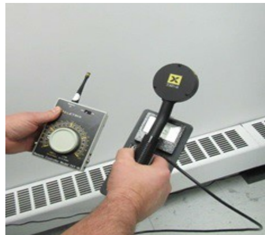
Simulated pancake probe and radiofrequency remote control
