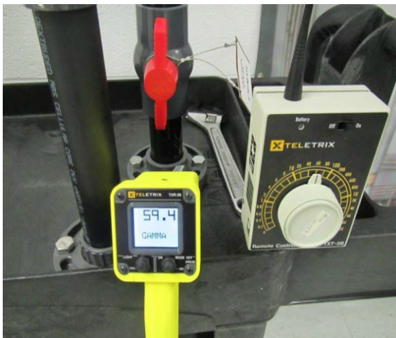
Simulated gamma meter and radiofrequency remote control
