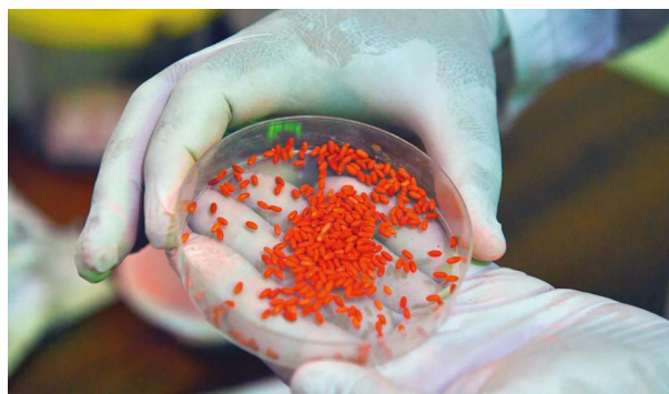
The Mediterranean Fruit Fly is successfully controlled in Jordan through the application of the sterile insect technique (SIT). In this photo, the pupae weight, percent emergence of sterile adult flies and flight ability are checked at the SIT Emergence Facility in Jordan Valley. (Photo: D. Calma/IAEA)
