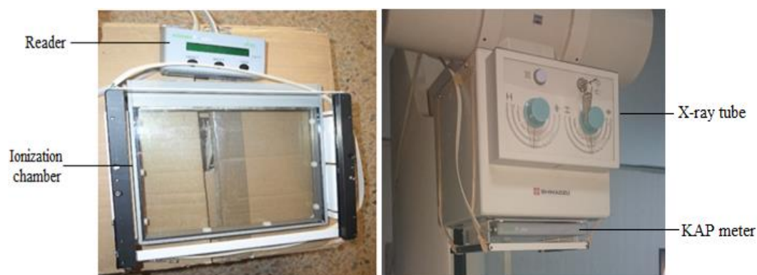
FIG. 1. KERMA X-plus iba dosimeter (KAP meter) on an X-ray tube
