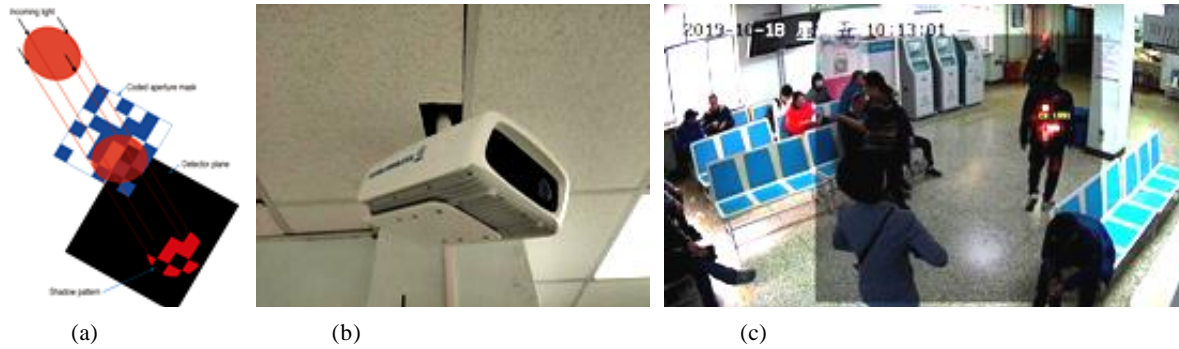
FIG. 1. Visual&auditory radiation detection and alarm system: (a) coded aperture imaging principle; (b) detector appearance and ceiling installation in Beijing Cancer Hospital; (c) an alarming case of a radioactive patient
