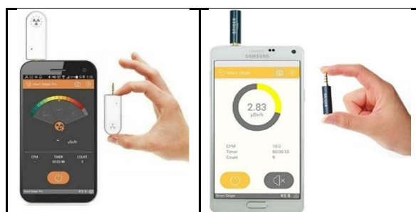
FIG. 26. Images of commercial Personal Radiation Detector plugged into smartphone as example.
