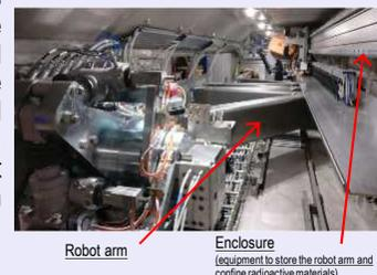
Robot arm Enclosure (equipment to store the robot arm and confine radioactive materials)
