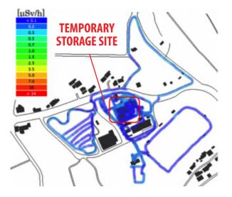
Radiation monitoring near a temporary storage site in the Nakadori region as an example of using walking survey.
