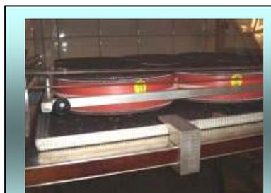
**Figure 17. Feeding plate fixed with aluminium clips.**
