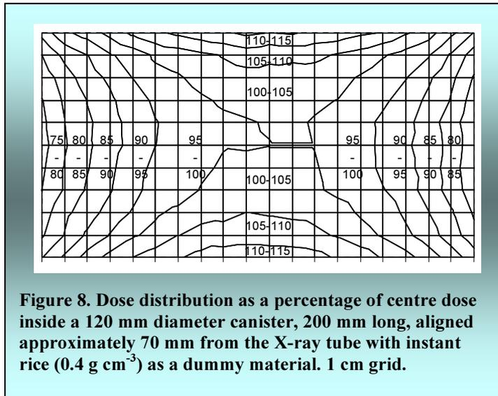
**Figure 8.** Dose distribution as a percentage of centre dose inside a 120 mm diameter canister, 200 mm long, aligned approximately 70 mm from the X-ray tube with instant rice ( $0.4 \text{ g cm}^{-3}$ ) as a dummy material. 1 cm grid.
