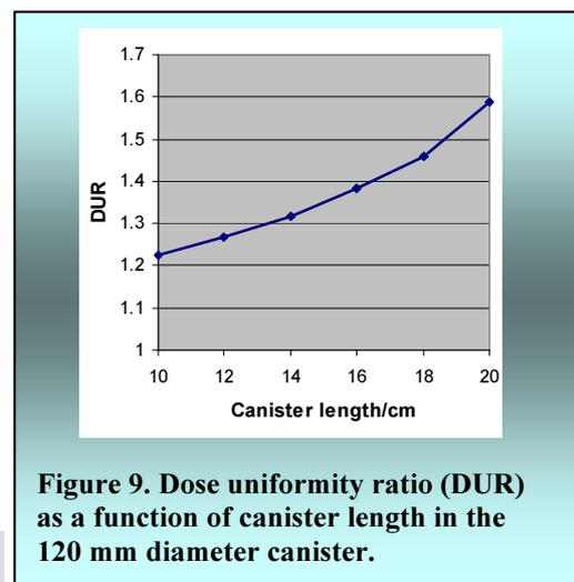
**Figure 9.** Dose uniformity ratio (DUR) as a function of canister length in the 120 mm diameter canister.
