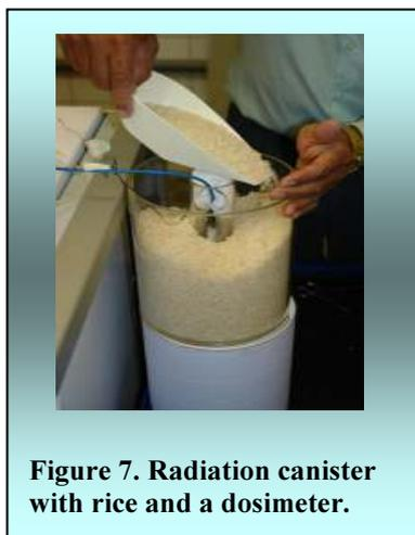
**Figure 7. Radiation canister with rice and a dosimeter.**
