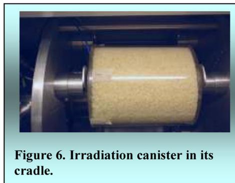
**Figure 6. Irradiation canister in its cradle.**
