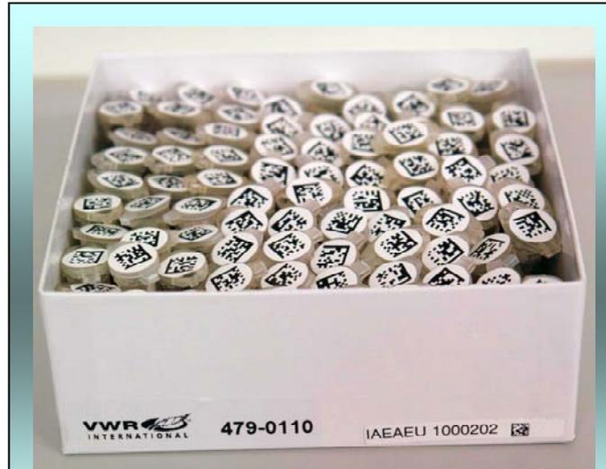
Figure 18. Individual tubes, storage boxes and freezer shelves are bar coded with a two-dimensional code to make sample identification and location simple.
