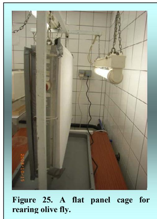
Figure 25. A flat panel cage for rearing olive fly.
