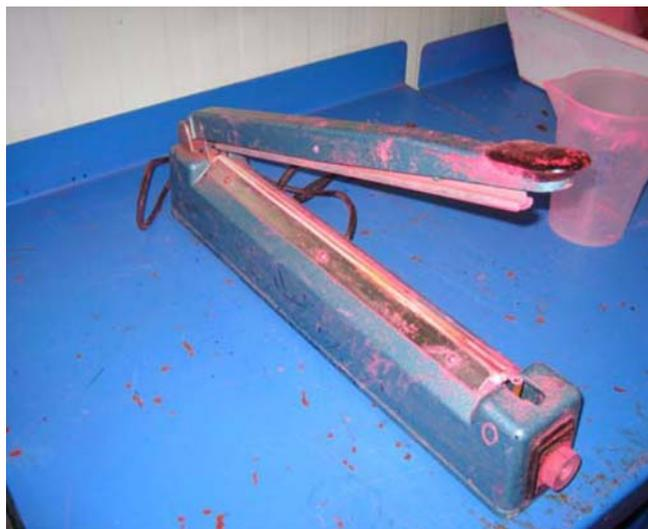
**FIGURE 6: Hypoxia is critical to reduce irradiation-induced damage during the sterilization process. Use a sealing machine to close plastic pupae ba, and standardize the post-sealing time to assure the desired level of hypoxia and humidity (QC9)**
