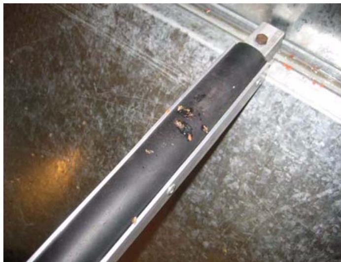
**FIGURE 5c:** Use of wire covered with tygon tubing reduces the damage to aluminum trays (L20).
