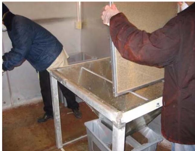
**FIGURE 5b:** Remove flies from the screens by hitting the aluminum trays against the metal bars.
