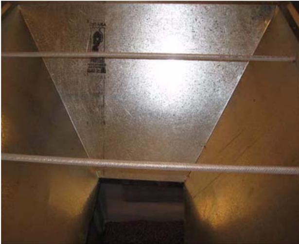
**FIGURE 5a:** The knockdown hopper has a solid metal bar that can damage the aluminum tray.
