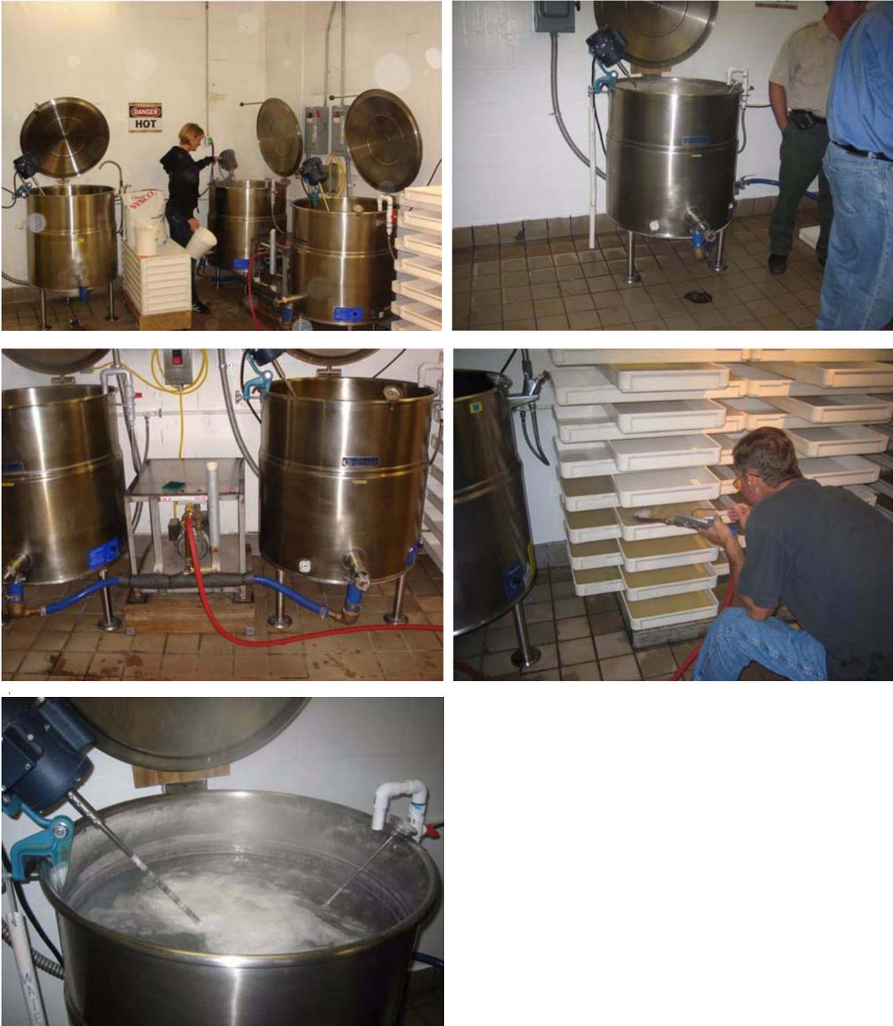
**FIGURE 3: Using mechanical blenders for adult diet preparation maintains the emulsion in continuous motion within the kettle, simplifies the process, and reduces labor time (L15, L16). Pump the liquid from the kettle directly into the fiberglass trays instead of using buckets to pour to reduce risk of serious injury to workers.**
