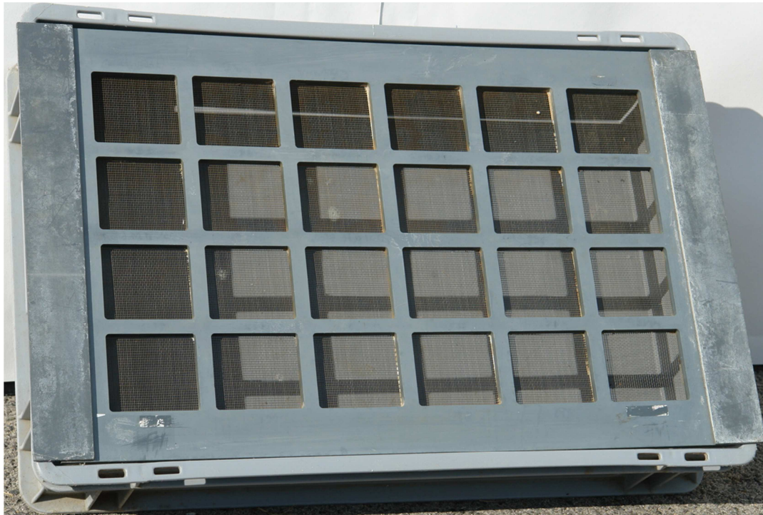
Photograph 2. Support platform sitting on top of test tank.
