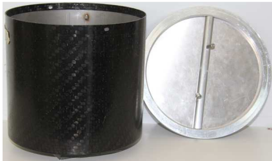
Figure 3: Sample canister and the cover, the interior of the canister is lined with a steel film to harden the X-ray beam.
