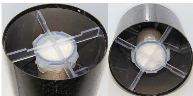
Figure 6b: Seed samples packed inside a sample container with adaptors to set inside the RS 2400 standard canister.
