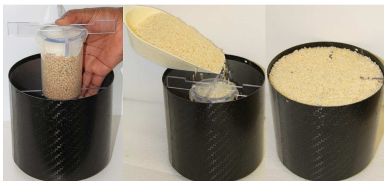
Figure 10: The prepared sample container is placed inside a standard RS 2400 canister where it is fixed in position by adaptor brackets. The space between the sample container and the canister is filled with instant cooking rice.
