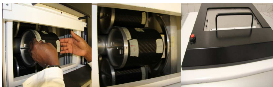
Figure 12: Placement of canister in Irradiator and closing the chamber.
