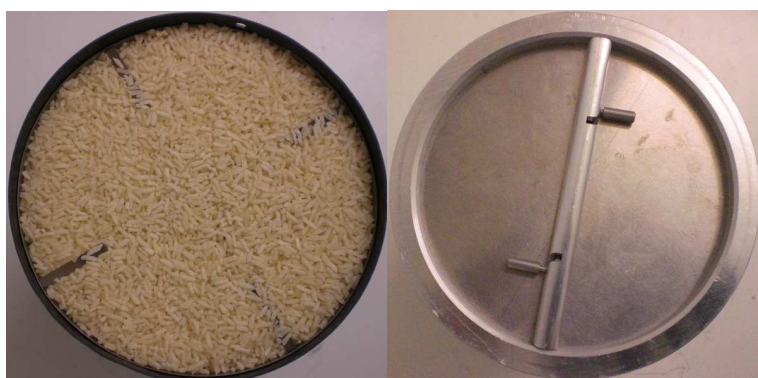
Photograph 11: Canister of samples with spare volume filled with by instant rice and cover canister by side.
