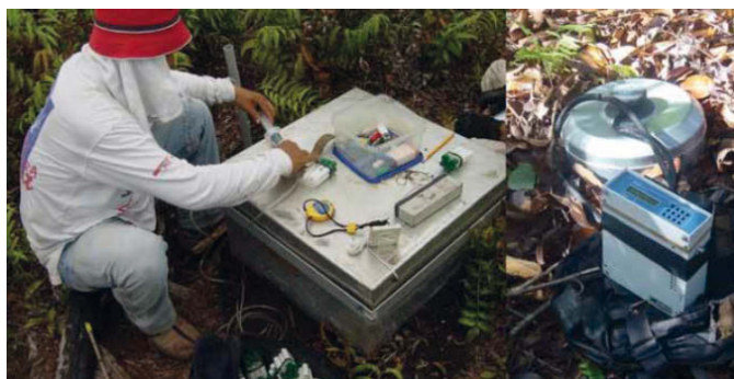
FIGURE 3. Closed chamber measurements being made in the field; large static chamber (left) and dynamic chamber and CO 2 analyzer (Page et al. , 2011).
