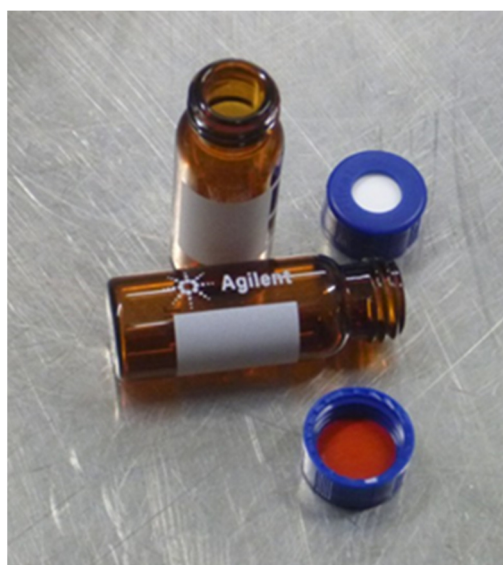
Figure 6: Screw cap 2-ml vials. The cap is fitted with a Teflon-coated silicon-rubber septum.
