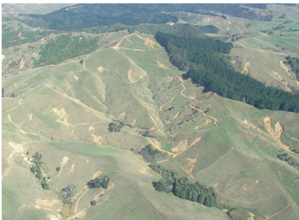
Figure 9: A small watershed in pasture with multiple land slips. The CSSI technique is not needed to identify where the sediment is coming from as the sources are obvious. Sediment transport from this sub-catchment may be a point source for a larger watershed.
