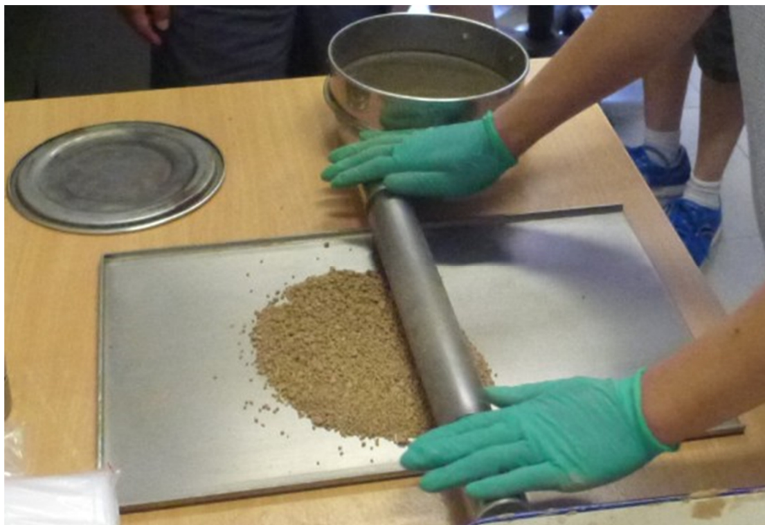
Figure 18: Lumps in the sample can be crushed with a steel roller on a steel tray to reduce the particle size to <2 mm. Crushing with a roller produces less very fine material than grinding.
