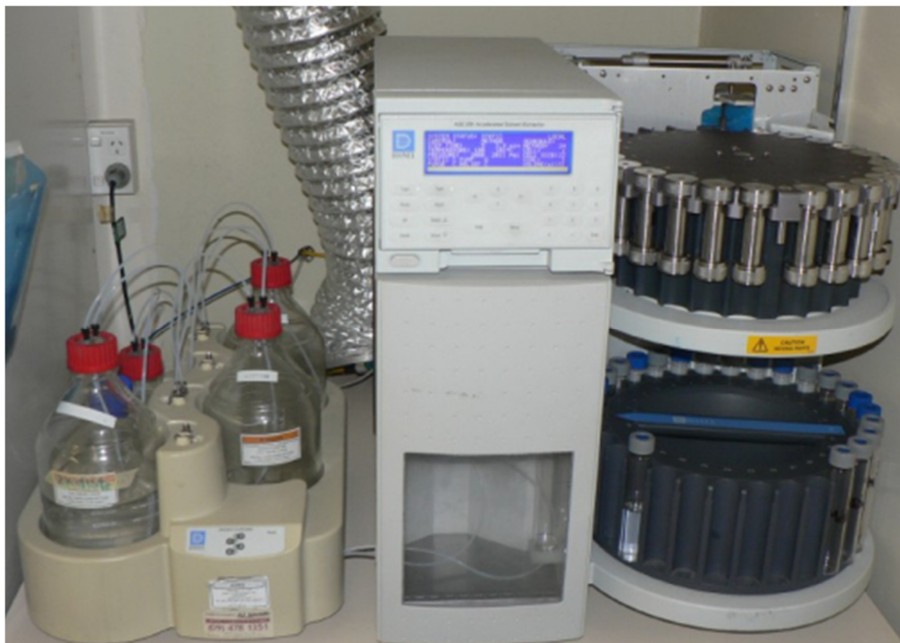
Figure 19: Dionex ASE 200 accelerated solvent extractor with load (sample) cells in the upper carousel and the extract collection vials in the lower carousel.
