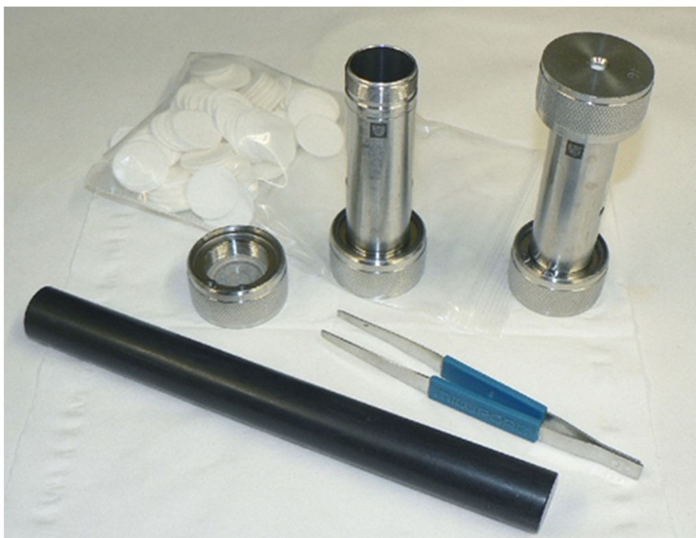
Figure 20: Two sample cells, one with the upper end cap off and showing the PEEK seal inside the end cap. The O-ring seal is located in the centre of the outside of each end cap and is visible in the top of the fitted end cap. The dark patch on the tubular body indicates the top. The filter pads (in plastic bag) fit tightly inside the cell body and need to be pushed down to the bottom of the cell with the assembly rod (black). Use smooth-tipped forceps to handle the filters.
