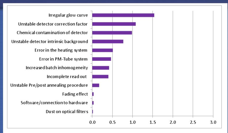
Figure 39. Most important sources of error for thermoluminescence dosemeters (TLDs)
