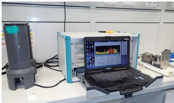
Figure 2: COMPUCEA (Combined Procedure for Uranium Concentration and Enrichment Assay) for uranium enrichment and assay measurement at NML.
