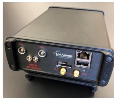
Figure 2: New Low-Current Data Acquisition Module (UDCM) selected by the UMS Team, developed by LANL and manufactured under license.
