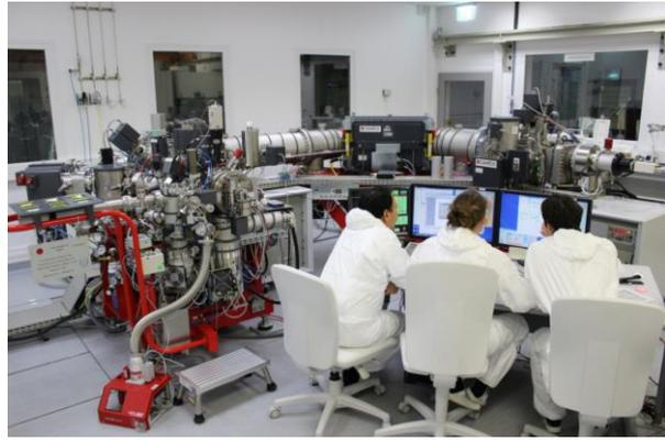
Figure 2: The regular replacement of ageing analytical equipment (like the ICP-MS on the left and the LG-SIMS on the right) is key to independently verifying nuclear activities impartially and on time.
