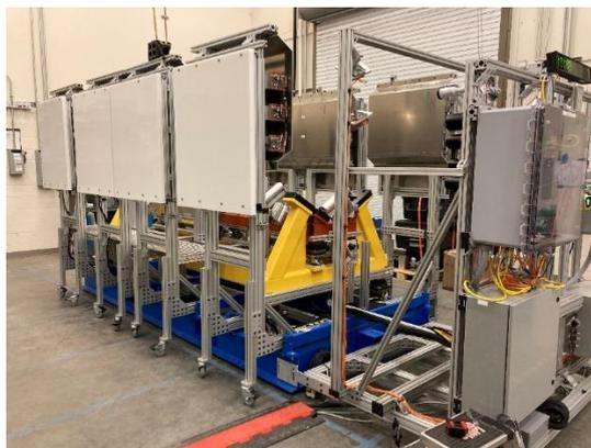
Figure 1: UCVS: Mechanical frame showing where the cylinders will be seated (yellow frame) and all surrounding slab detectors for UF<sub>6</sub> characterization.
