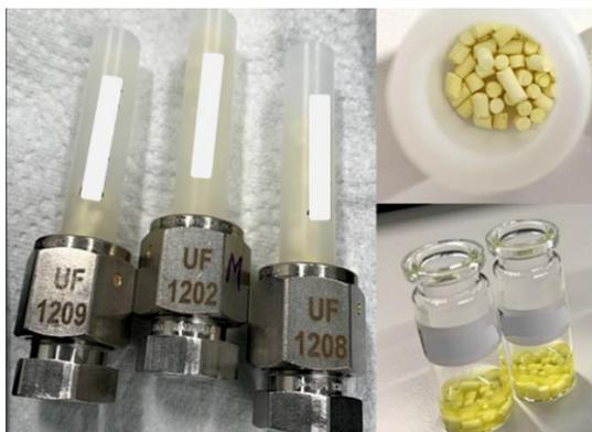
Figure 5: ABACC Cristallini samples of UF<sub>6</sub>.
