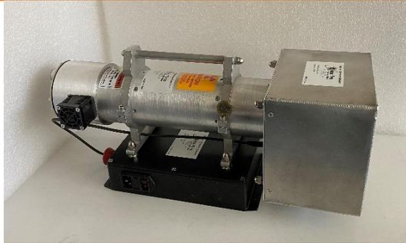
Figure 1: nGen-350 D-D neutron generator for use as a neutron interrogation source with FNCL.
