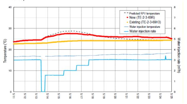
Figure. Changes in PRV bottom temperature during the test to suspend water injection
