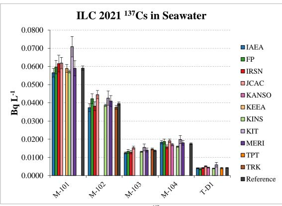
FIG. 5 Activity concentrations of <sup>137</sup>Cs in seawater samples.
