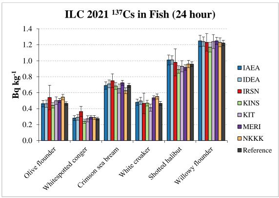
FIG. 12. Massic activities of <sup>137</sup>Cs in fish samples (24-hour measurement time).
