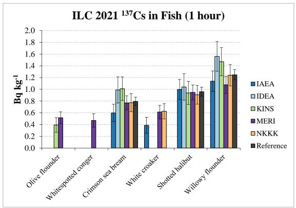
FIG. 11. Massic activities of <sup>137</sup>Cs in fish samples (1 hour measurement time).
