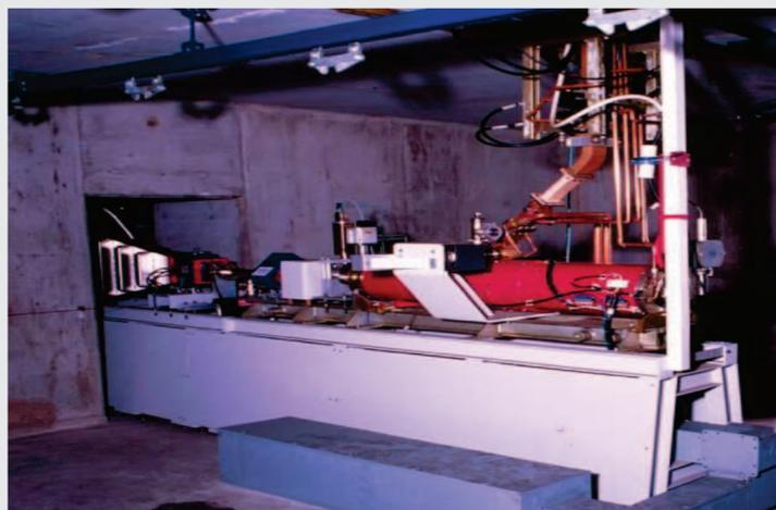
An example of an accelerator based industrial irradiator. Note the thick (approx. 2 m) concrete walls which are required to shield against the high doses inside the irradiator.
