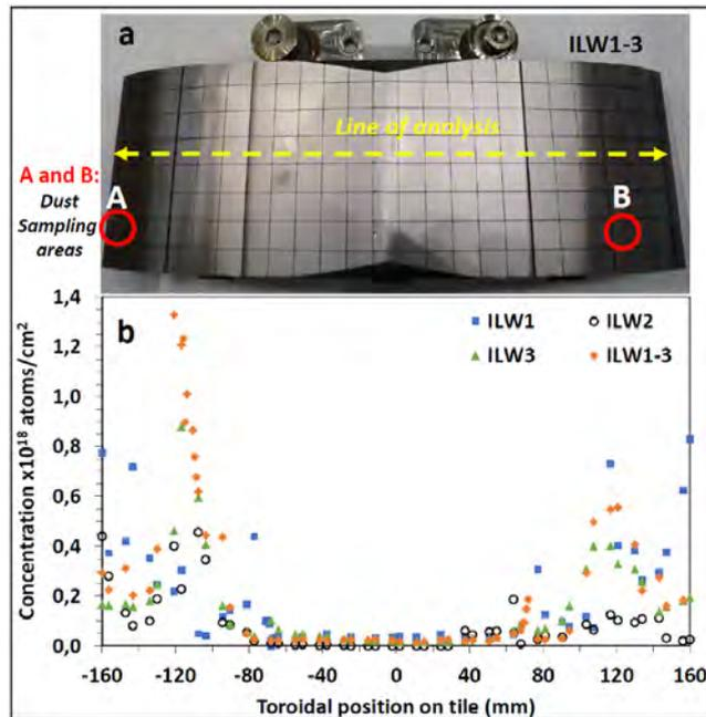
Fig. 1. (a) Castellated beryllium mid-plane IWGL tile after exposure in JET; (b) Deuterium areal concentrations at mid-plane measured after consecutive campaigns and after all three campaigns ILW1-3; data reproduced with permission of copyright holder UKAEA and author [2,3].
