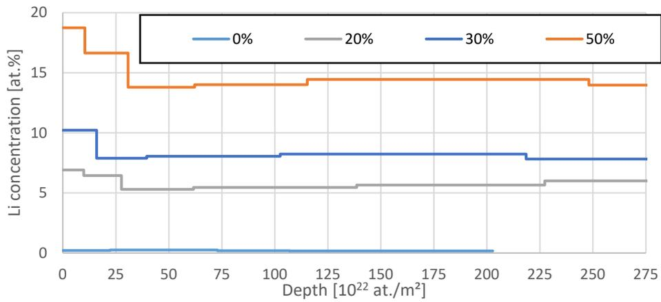
FIG 2: Comparison of the Li depth profiles. The first  $\sim 6 \mu m$  are enriched with Li. The region  $> 200 \cdot 10^{22}$  at./ $m^2$  has to be considered with care due to the dominance of the pile-up signal in this deep region.
