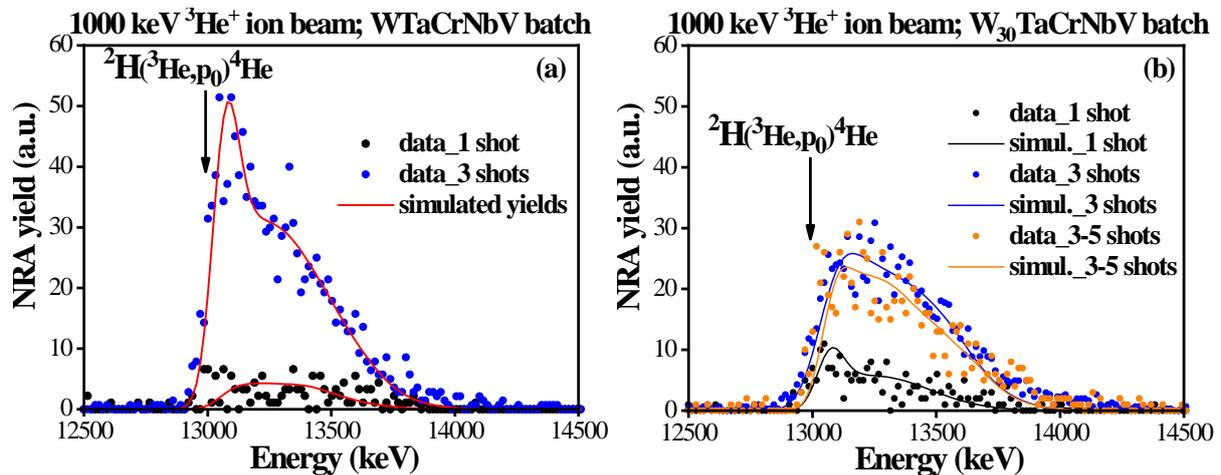
FIG. 2: NRA spectra and corresponding fit lines achieved from the elemental quantification using the NDF code [6]: (a)  $W_{20}Ta_{20}Cr_{20}Nb_{20}V_{20}$  and (b)  $W_{30}Ta_{17.5}Cr_{17.5}Nb_{17.5}V_{17.5}$  alloy.
