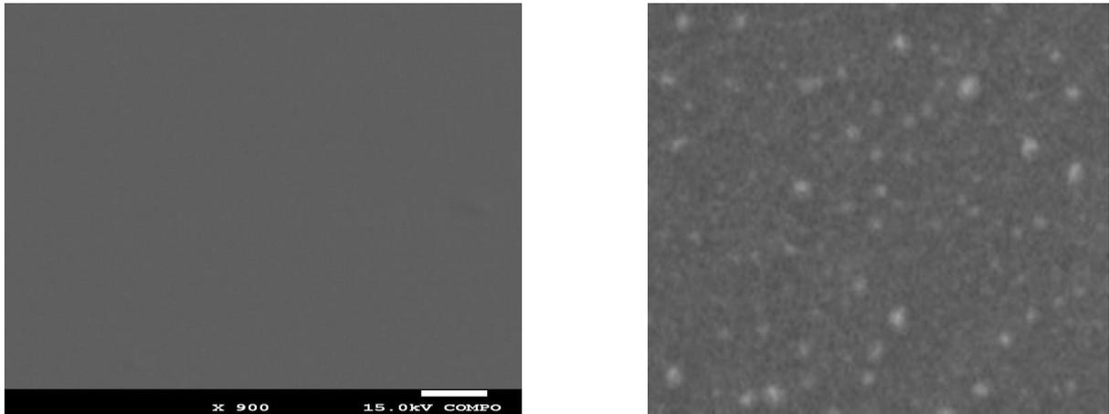
*FIG.1. SEM images of a implanted TiO<sub>2</sub> film before (left) and after annealing (right) at 500 °C, 15 min.*
