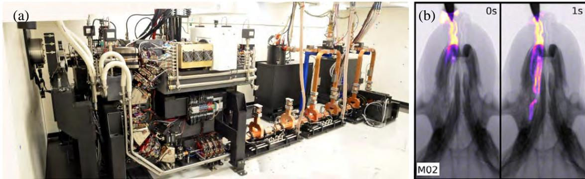
*FIG. 2. (a) Photograph of the Lyncean Compact Light Source. (b) Example of a dynamic in vivo imaging application from the Munich Compact Light Source, showing delivery of liquid instillations to the nose of a mouse (adapted from [7], Creative Commons License).*
