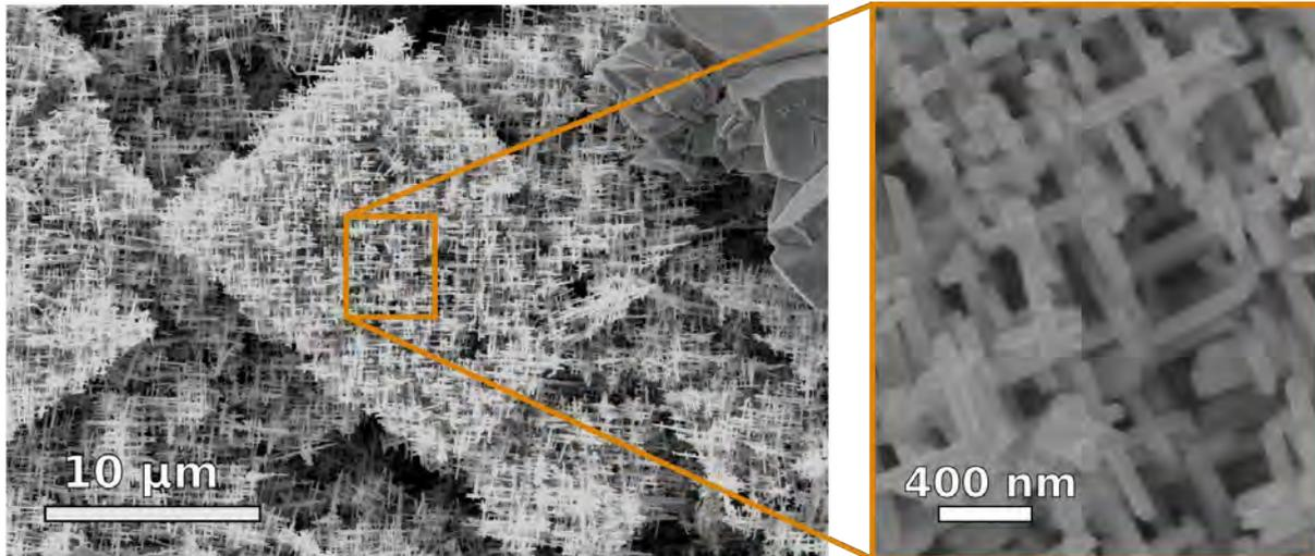
*Fig. 1 SEM image of a Bi nanowire network consisting of  $1.4 \times 10^9$  wires per  $\text{cm}^2$  with a wire diameter of  $\sim 100$  nm together with a close-up illustrating the wires interconnected within the network.*
