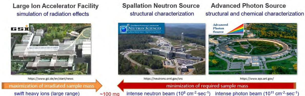
FIG. 1. Swift heavy ions with large penetration depths are required to produce sufficiently large quantities of homogeneously irradiated materials ( $\sim 100 \text{ mg}$ ) that can be analysed by spallation neutron and synchrotron X-ray probes.
