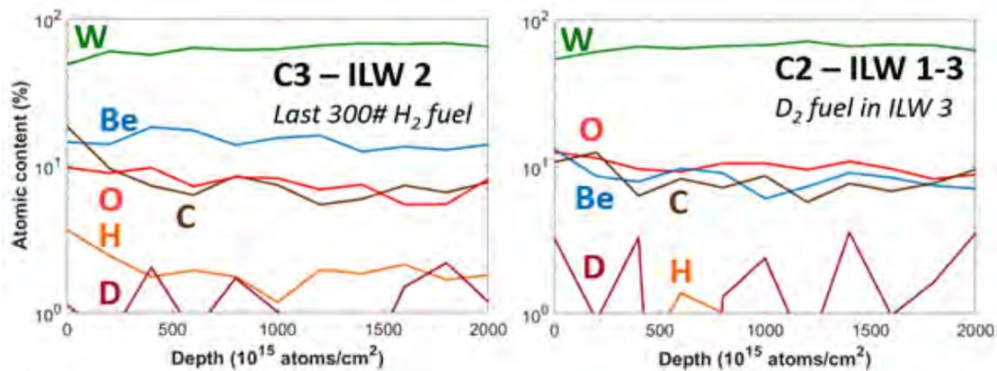
FIG. 1. HI-ERDA depth profiles of elemental composition on W samples from neighbouring positions C3 and C2, retrieved after ILW-2, which finished off with 300 shots of  $\text{H}_2$ , and ILW-3, which finished with  $\text{D}_2$  fuelling. The total hydrogen isotope retention is  $6.7 \times 10^{16}$  and  $5.3 \times 10^{16} \text{ cm}^{-2}$ , respectively.
