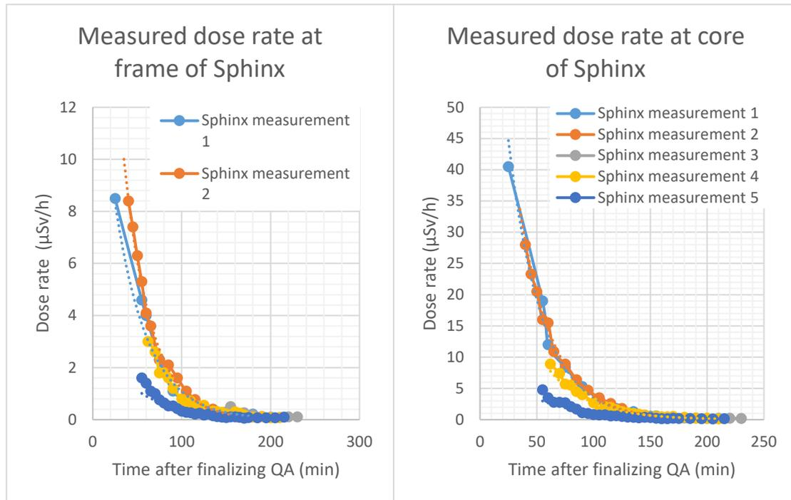
*Spectrum-based measurements performed on activated metallic parts of the accelerator show the presence of Co-57 and Co-60. Dose rates at contact can vary significantly, from a few μSv/h up to 1 mSv/h for the most activated components.*
