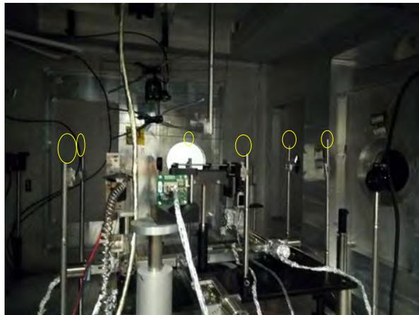
*FIG. 1. Position of EBT3 detectors inside the interaction chamber for radiation isodose measurements*
