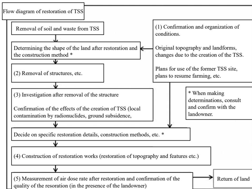
Figure 6. Flow diagram of restoration of TSS<sup>2</sup>
