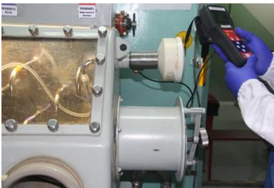
Sampling box (before modification by the plant): O 2 /H 2 manual measurement
