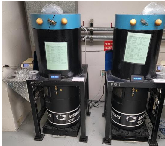
Figure 1: Mobius Recycler Installed Underneath Intrinsic Germanium Detectors
