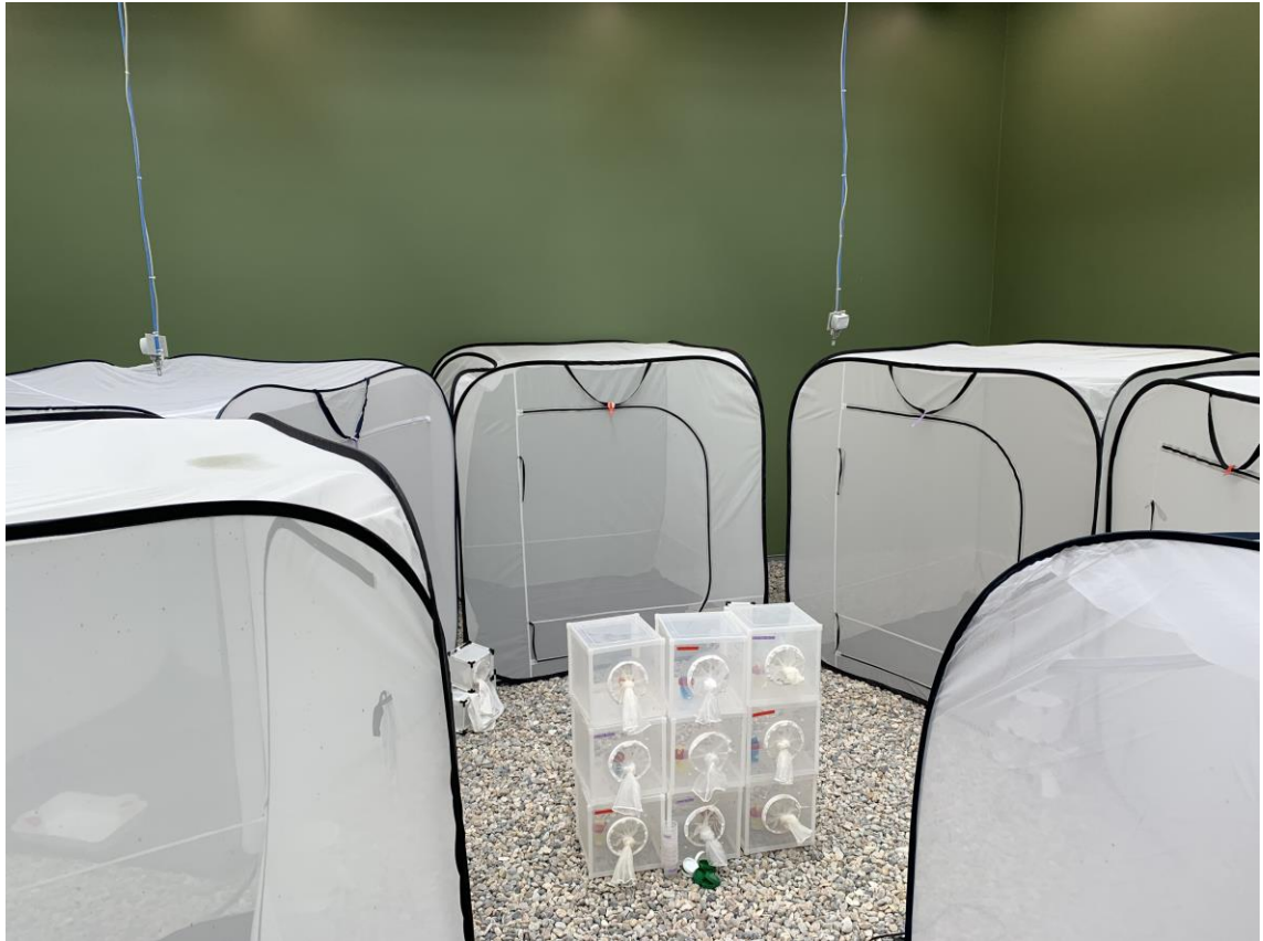
Figure 2B. Example of a semi-field cage experiment setting: Nine 30×30×30cm control cages (irradiated (low, high doses) and non-irradiated males only) and six large competition cages, each containing 100 males (irradiated and/or non-irradiated) and 100 virgin females. Low and high stand for low irradiation (inducing more than 99% sterility) and high irradiation dose (100Gy more that the low dose)
