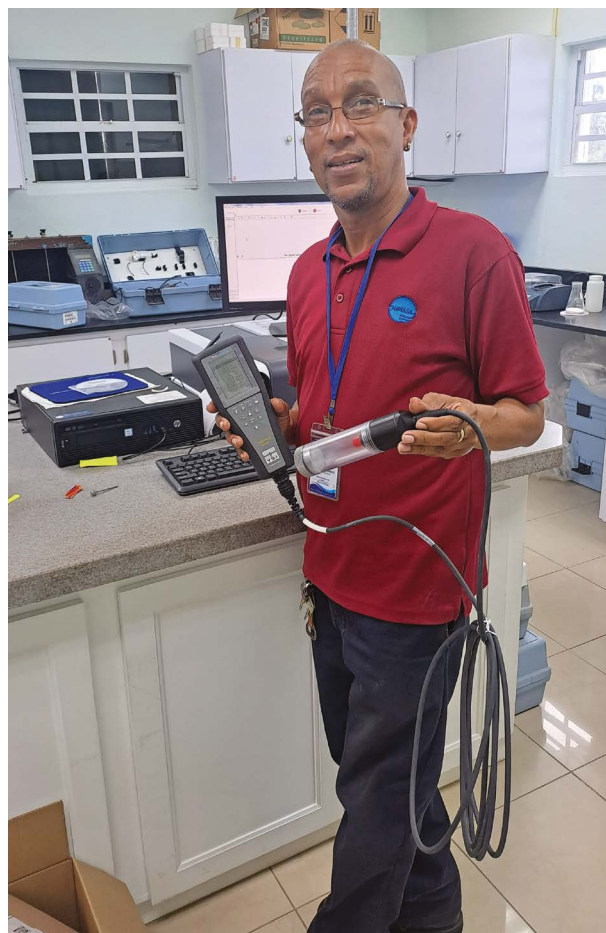
A technician at the National Water and Sewerage Authority holding a YSI PRO -QUATRO handheld meter – used to measure dissolved oxygen, electrical conductivity, ammonium, pH and nitrate. (Photo: D. Gabriel / National Water and Sewerage Authority, Grenada)
