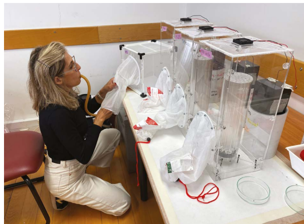
In a laboratory, adult sterile male mosquitoes are transferred from a net cage to a FAO/IAEA Flight Test Device (FTD) for quality control purposes. (Photo: H. Osório)
