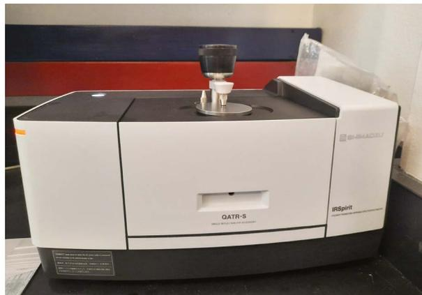
Infra-red spectrometer for microplastic monitoring, provided by the IAEA to the Institute of Marine Affairs, as part of the support to strengthen the institution's analytical capabilities in relation to the marine environment. (Photo: I. Tolosa/IAEA)
