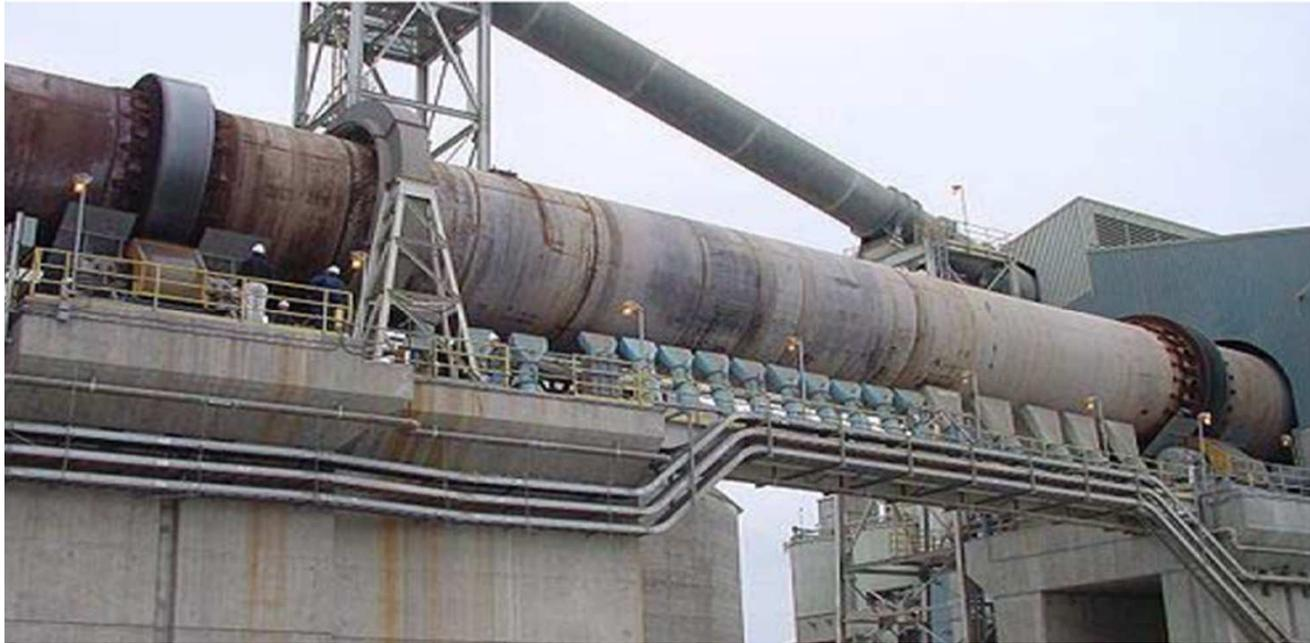
RTD of the homogenized fine crude mixture has been determined in different zones of a **rotary kiln**.
