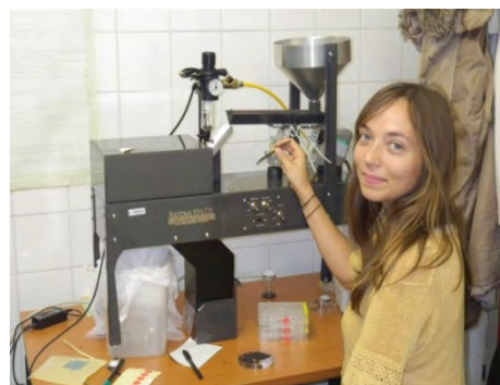
FIG 3: Ms Zelda Moran sorting pupae of Glossina palpalis gambiensis using the new near infrared tsetse pupal sorter
