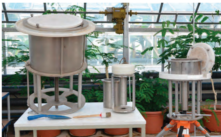
FIG. 1: Different diameters of the Fine Increment Soil Collector (FISC)
