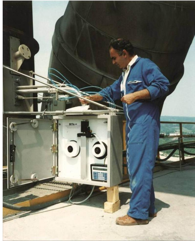
Measurement of atmospheric dust concentration ( $\beta$  absorption -  $^{14}\text{C}$ )
