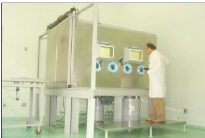
Figure H7. Hot Cell for Dismantling Nuclear gauges
