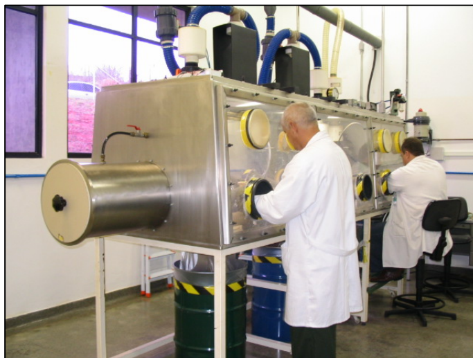
Figure H.1. Lightning rod dismantling glove-box
