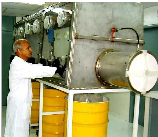
Figure H6. Lightning rod dismantling Facility
