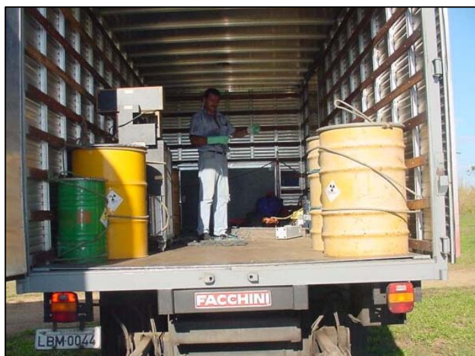
Fig J.2. Type A waste containers
