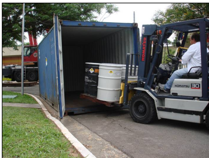
Figure I.1. Container loading with encapsulated sources
