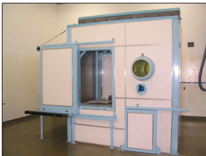
Figure H.2. Hot cell designed to handle sources (under construction)
