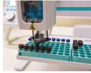
6 The process of taking LAS measurements of water stable isotopes is made more efficient through the use of an auto-sampler. Automating processes not only save time and effort for the scientists, but also insures greater consistency in procedure for a very sensitive technique.
