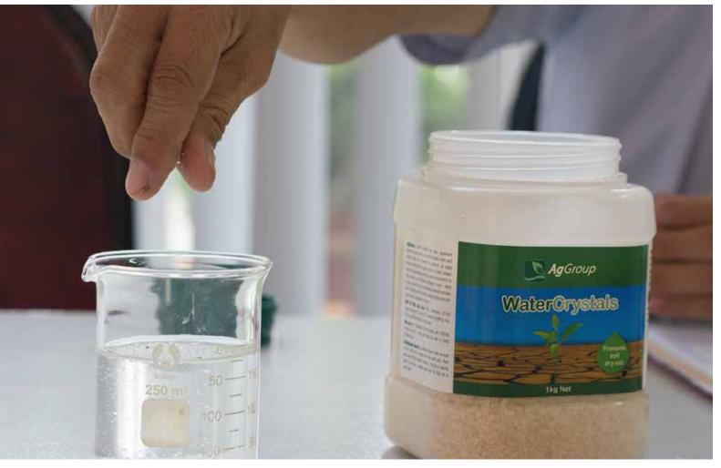
Through the power of irradiation to break and create chemical bonds, the natural polymer cassava starch is used to make super water absorbents (SWA), 1kg of which can absorb and hold 200 litres of water and release it slowly over time. Placed in the soil near plants' roots, SWA can be used where there is little rain or frequent drought. After 9 months the crystals, which resemble sugar crystals, completely disintegrate, leaving no residue.
