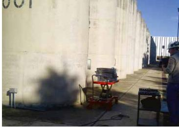
4 PUI funds are also being used to support research on the very long term storage performance of spent nuclear fuel and related storage system components. This also includes research into the long term integrity of dry storage concrete systems. Using an experimental setup of LaBr3 and Nal(Tl) gamma detectors, experts check the confinement integrity of the spent fuel and the structural integrity of the reinforced concrete silos at Embalse NPP's dry storage, Argentina. (Photo: CNEA/NA-SA)
