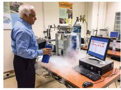
5 One of the ways scientists conduct carbon isotopic assays in water, rocks, CO<sub>2</sub> and dissolved carbon is through laser absorption spectrometry (LAS). As its name implies, LAS uses lasers to determine the types and concentration of isotopes it has by measuring the way it interacts with a test subject.
