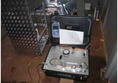
4 Isotopic techniques help understand surface water movement and inter-action with groundwater, dam leakages, and the impact of climate change on water resources development and management. Pictured is a sampling device for measuring noble gases and isotopes in groundwater.
