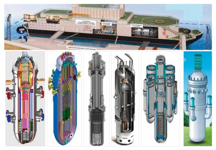
4 There is growing interest in small and medium sized nuclear power reactors (SMRs), partly because they allow smaller, more flexible and incremental investment over time. 'Small' means fewer than 300 MW(e), 'medium sized' means between 300 MW(e) and 700 MW(e). There are approximately 45 innovative SMR concepts at various stages of research and development. This diagram illustrates some of the SMR concepts deployable within the next decade.
