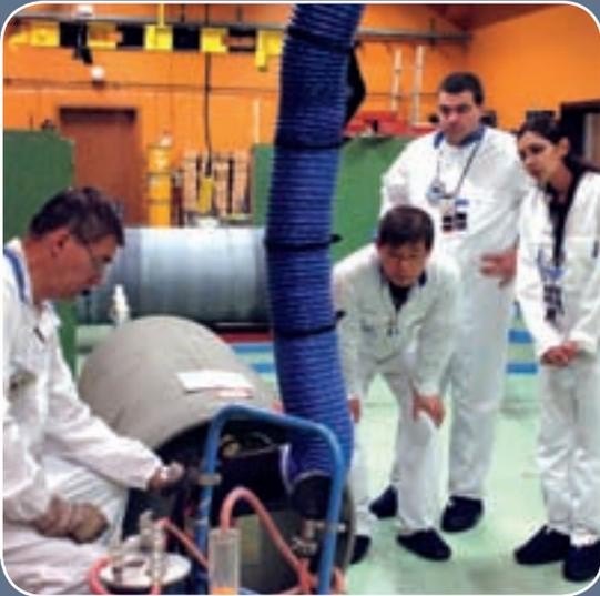
**7** Another step for inspectors is to verify levels of enrichment during the uranium conversion process. Here inspectors observe a plant operator carefully extracting a UF<sub>6</sub> sample to be analyzed for isotopic composition.
