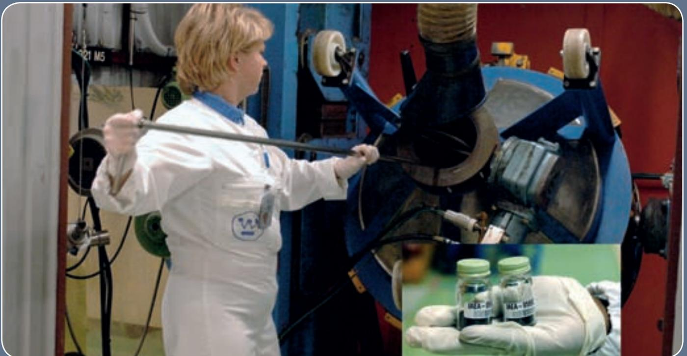
**9** A facility operator carefully takes a sample from the tilted hopper. The powder sample is poured into two small glass bottles (inset).
