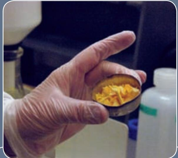
**8** The UF<sub>6</sub> sampling process ends up with concentrated uranium dioxide, a form of "yellowcake". The sample is baked in a furnace for three hours to mimic the uranium conversion process. Thereafter, the sample is sent to the IAEA's Safeguards Analytical Laboratory in Seibersdorf, Austria, for analysis of enrichment levels.
