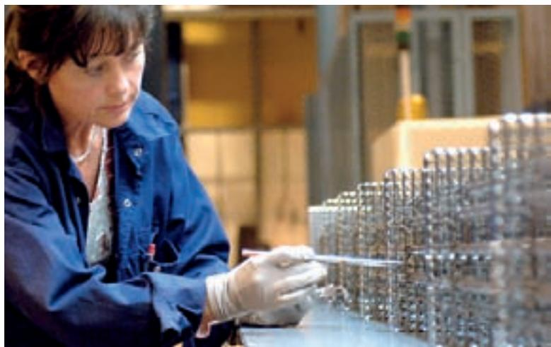
**Alternative initiatives to securing the nuclear fuel cycle are once again on the table. Here, at one of the final stages of fuel assembly, a technician checks nuclear fuel rods.** Photo: Dean Calma
