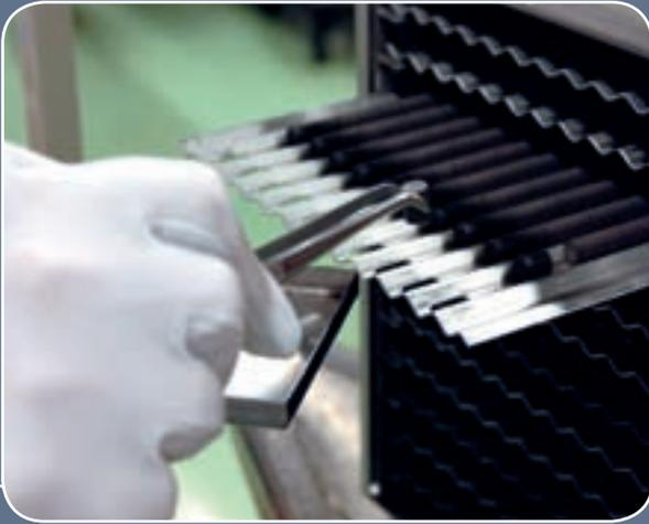
**10** Metal boxes hold trays of finished fuel pellets. Each pellet, slightly larger than a pencil eraser, contains enriched uranium dioxide that will be used at nuclear power plants.
