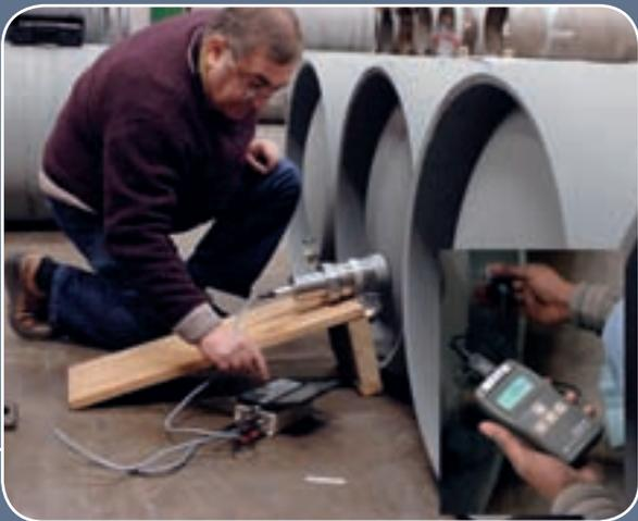
**5** Checking the cylinder is one thing. Checking what's inside is another. Inspectors rely on sophisticated instruments — such as germanium detectors and sodium iodide, pictured here, to detect enrichment levels — most enriched material emits gamma rays. These tools of the trade help inspectors verify the accuracy of the facilities' records.
