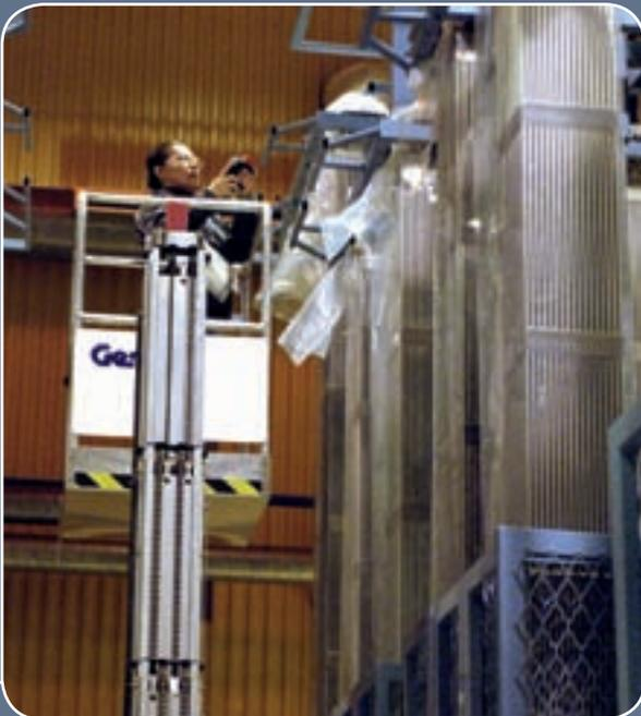
**12** Going up to the source is sometimes the only way to access the assemblies for critical measurements. In this case, an inspector is hoisted into the air on a crane to get an active length measurement.
