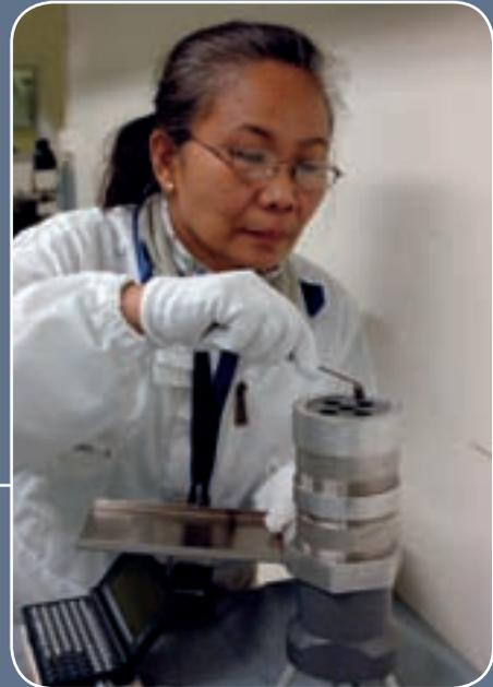
**11** An inspector verifies the pellet's enrichment using an instrument called a Mini-Multichannel Analyzer that attaches to a palm-sized computer.
