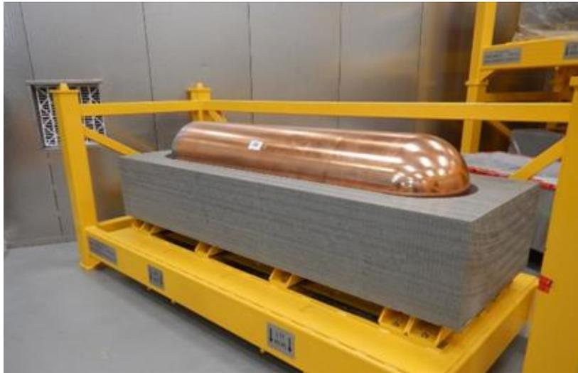
The NWMO is also developing non-destructive examination techniques and custom equipment to inspect the UFCs following the various stages of fabrication, such as welding, copper coating and machining. These inspections will ensure that UFCs meet the required specifications.
