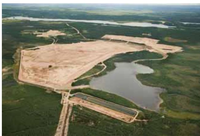
**Figures 7.3 (a) and (b)** – Photographs show the TMA during operation and after decommissioning but prior to the re-vegetation becoming established.
