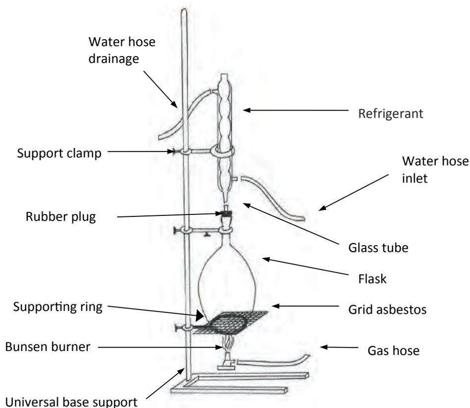
The equipment must be set up by placing the refrigerant in the holder and holding it vertically with a clamp and then connecting the coolant to hoses that convey the water. The first hose is placed in the lower projection of the coolant and linked to a water source; in the other projection, the upper hose is the drain. The bottom of the refrigerant must be attached to a glass tube, and the latter is attached by means of a rubber plug or ball to the flask containing the solution.
