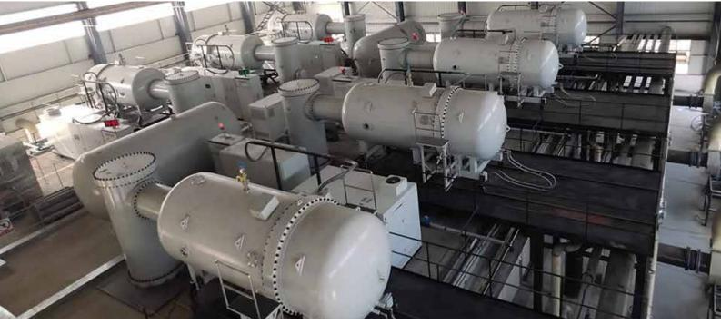
Seven electron accelerators treat printing and dyeing wastewater at Guanhua Knitting Factory. (Photo: Nuclear and Energy Technology Institute, Tsinghua University)
