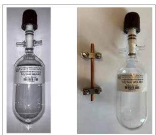
Reference materials are physical standards that are used to calibrate laboratory equipment. (Photo: IAEA)
