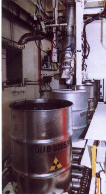
Fig. 4.6 View of a bituminisation line to condition liquid RAW
