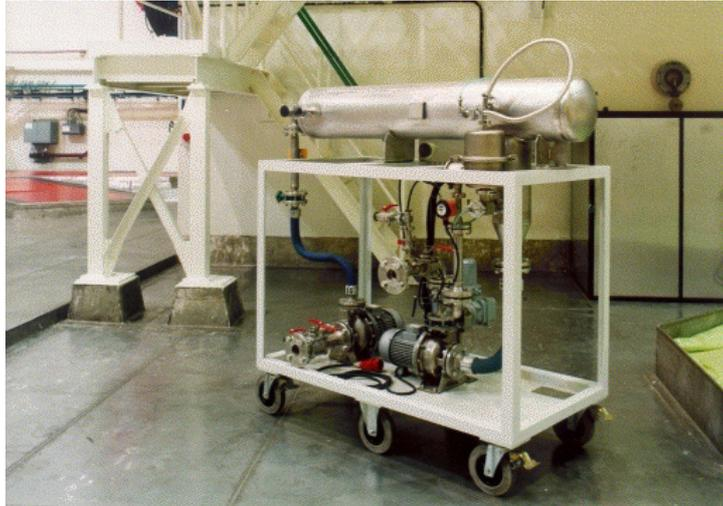
Fig. 7.4 Equipment for water re-flooding of CASTOR-440/84 cask.
