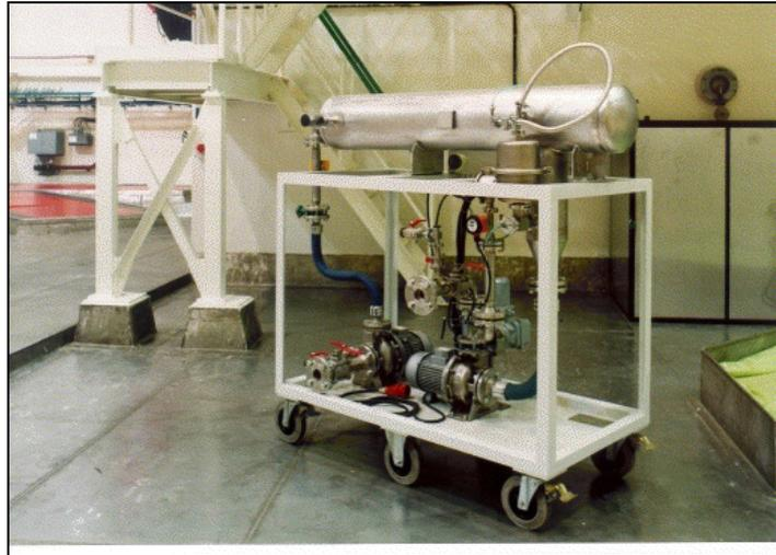
Fig. 7.4 Equipment for re-flooding of CASTOR-440/84 casks
