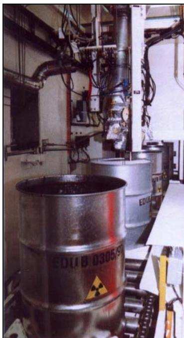
Fig. 4.5 View of a bituminization line to process liquid RAW
