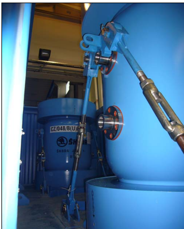
Fig. 9.1 Two ŠKODA VPVR/M casks in a transport ISO container
