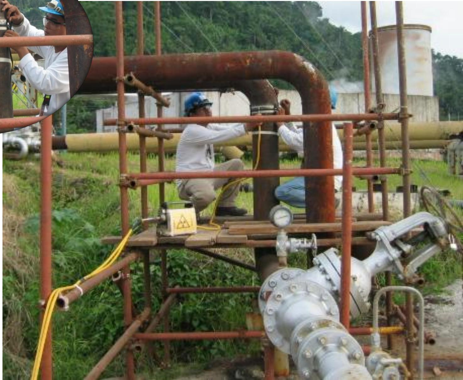
Radiographic testing of pipeline using Iridium-192 gamma source
