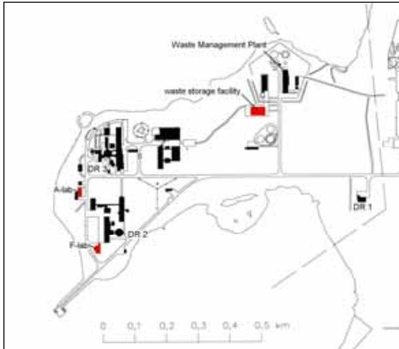
Figure 1. Map of Danish Decommissioning nuclear facilities and associated buildings at the Risø peninsula. Reactors: DR 1, DR 2, DR 3. New facilities: waste storage facility, A-lab, F-lab, and Waste Management Plant.
