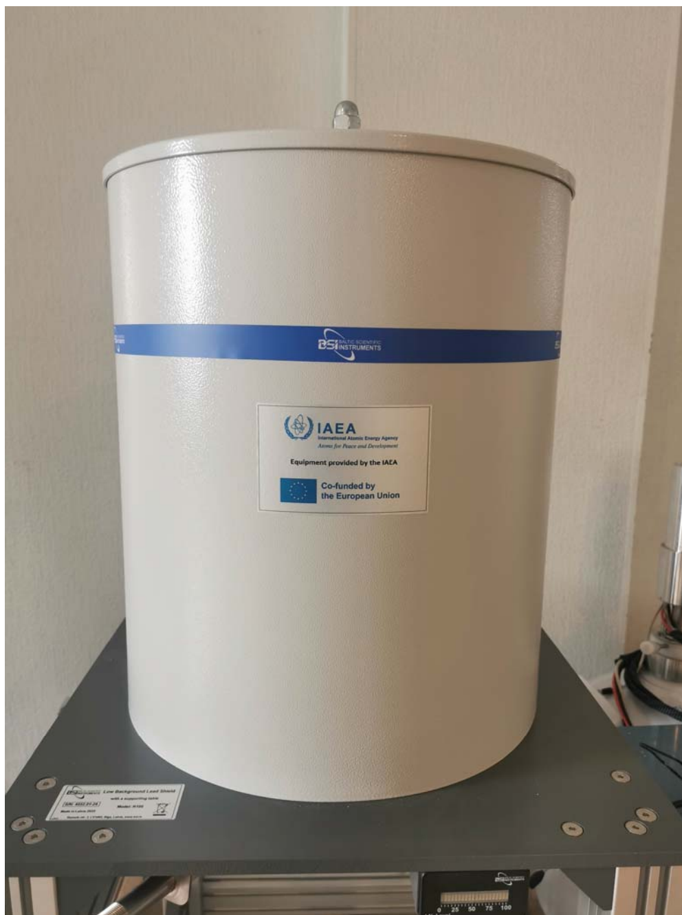
Gamma spectrometer with a high purity germanium detector delivered to the Rivne Regional Centre for Hydrometeorology, Ukrainian Hydrometeorological Centre and the Hydrometeorological Organizations of the State Emergency Service of Ukraine on 12 March 2025. (Photo: Rivne Regional Centre for Hydrometeorology)
