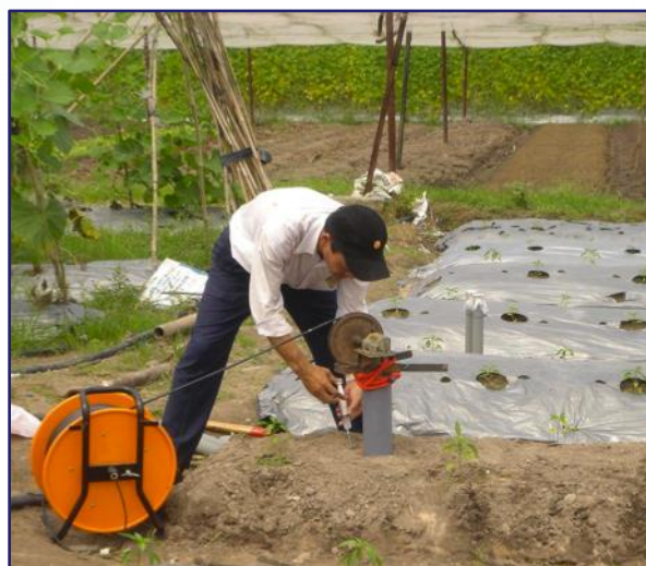
Iodine-131 was used to trace the infiltration of water in soil.
