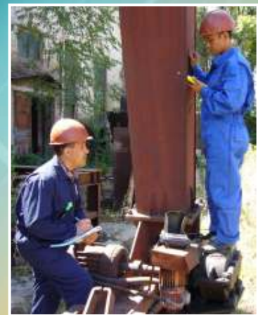
Thickness measurement using an NDT technique.
