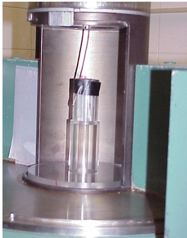
Figure 23. Three dosimeters in a cylindrical dosimeter holder on a stand are prepared for irradiation in a Gammacell. Thermocouples are used to measure the temperature throughout the irradiation, where the thermocouple junction is located inside the dosimeter holder next to the dosimeters. A black tape is used to hold the wires firm in position. The wires leave the irradiation chamber through the central access tube to the recording device situated outside the Gammacell.
