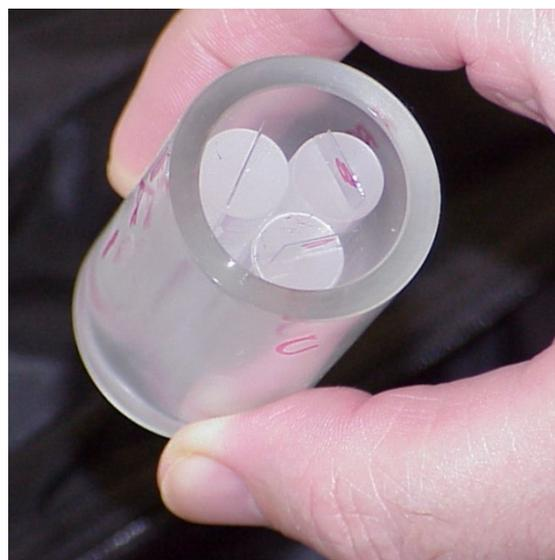
Figure 21. Three film holders with Gafchromic™ dosimeters are placed in a cylindrical dosimeter holder for irradiation in a Gammacell. Note that each film holder is placed so that the film is parallel (tangential) to the curved surface of the dosimeter holder. For a flat dosimeter holder, the film holders should be placed so that the films are parallel to the longer face of the dosimeter holder.
